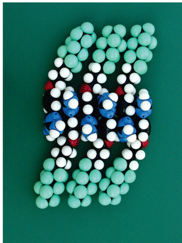
Figure 3. CPK model of the smectic A mesophase of the single-chain semiperfluorinated triazine 6 -[ 4 , 6 ].
